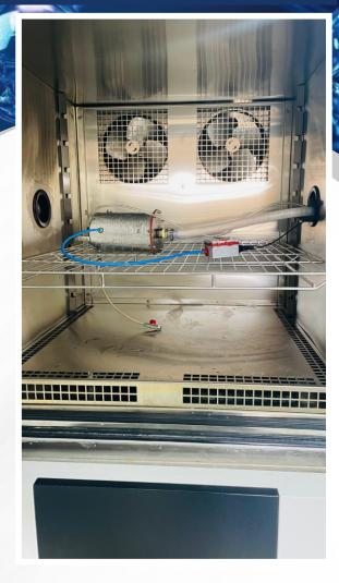
Envisys engineered a specialized climatic test chamber tailored for hydrogen sensor testing, incorporating stringent safety and control systems to meet high-performance requirements. This chamber includes an integrated inertization system to mitigate risks associated with hydrogen, a fire suppression system, and comprehensive gas and heat detection systems adhering to EUCAR safety standards.
